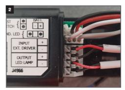
IN CERTAIN CIRCUMSTANCES THE PANEL USED WITH THIS EMERGENCY KIT MAY NOT OPERATE IN EMERGENCY, WHILE IT STILL MAY OPERATE IN MAINTAINED. IF THIS IS THE CASE AND THE GREEN LED IS LIT, IT WILL BE NECESSARY TO REVERSE THE POLARITY OF THE LOW VOLTAGE INPUT AND OUTPUT CABLES.
