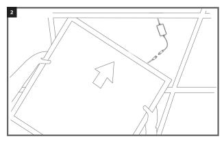
3. When the panel is through, orientate it horizontally and lower to rest onto the top of the tee bar on all four sides. Reconnect the mains supply once the panel is securely in position.
