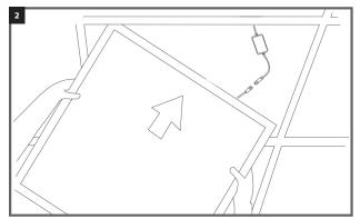
3. When the panel is through, orientate it horizontally and lower to rest onto the top of the tee bar on all four sides. Reconnect the mains supply once the panel is securely in position.
