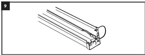
10. Connect the battery cell within the emergency kit and close the battery cell door.
